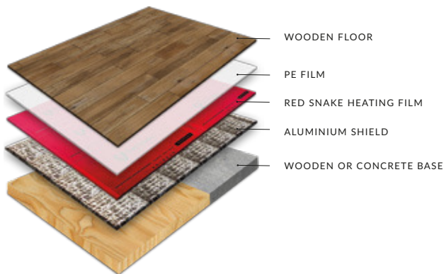
INSTALLATION ARRANGEMENT FOR PANELLED FLOORS
